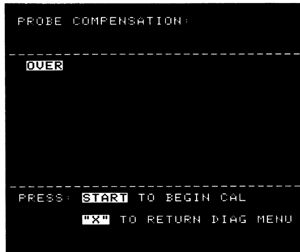
Figure 3-19. Display for External Clock Probe compensation.
