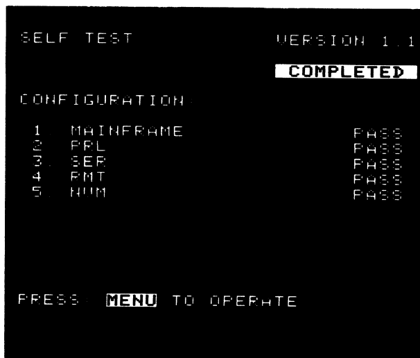
Figure 5-3. 318 Successful Power-up diagnostics display.
