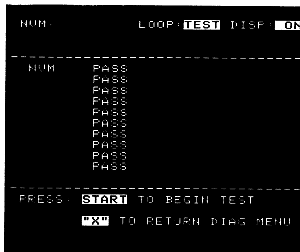
Figure 3-24. Display for the non-volatile memory test (NVM).
